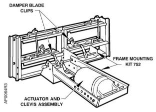
Figure 5. Two-section Damper.
