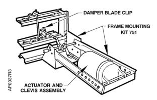
Figure 3. One-section Damper.
