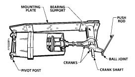
Figure 9. Extended Shaft Remote Mounting Assembly.
